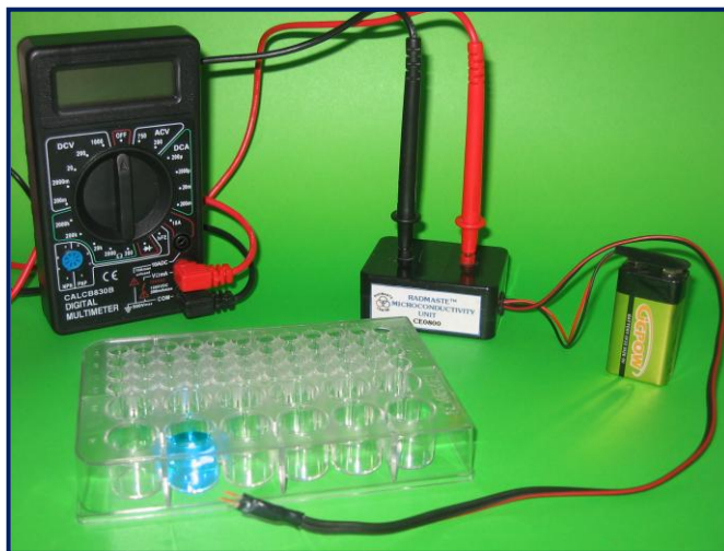
A Microconductivity Unit is available to measure conductivity of solutions in the comboplate of the GWK
