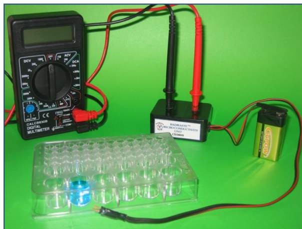
A Microconductivity Unit is available to measure conductivity of solutions in the comboplate of the GWK
